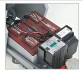
Easy access to onboard charger. Wet-acid batteries are standard. Gel batteries are optional
